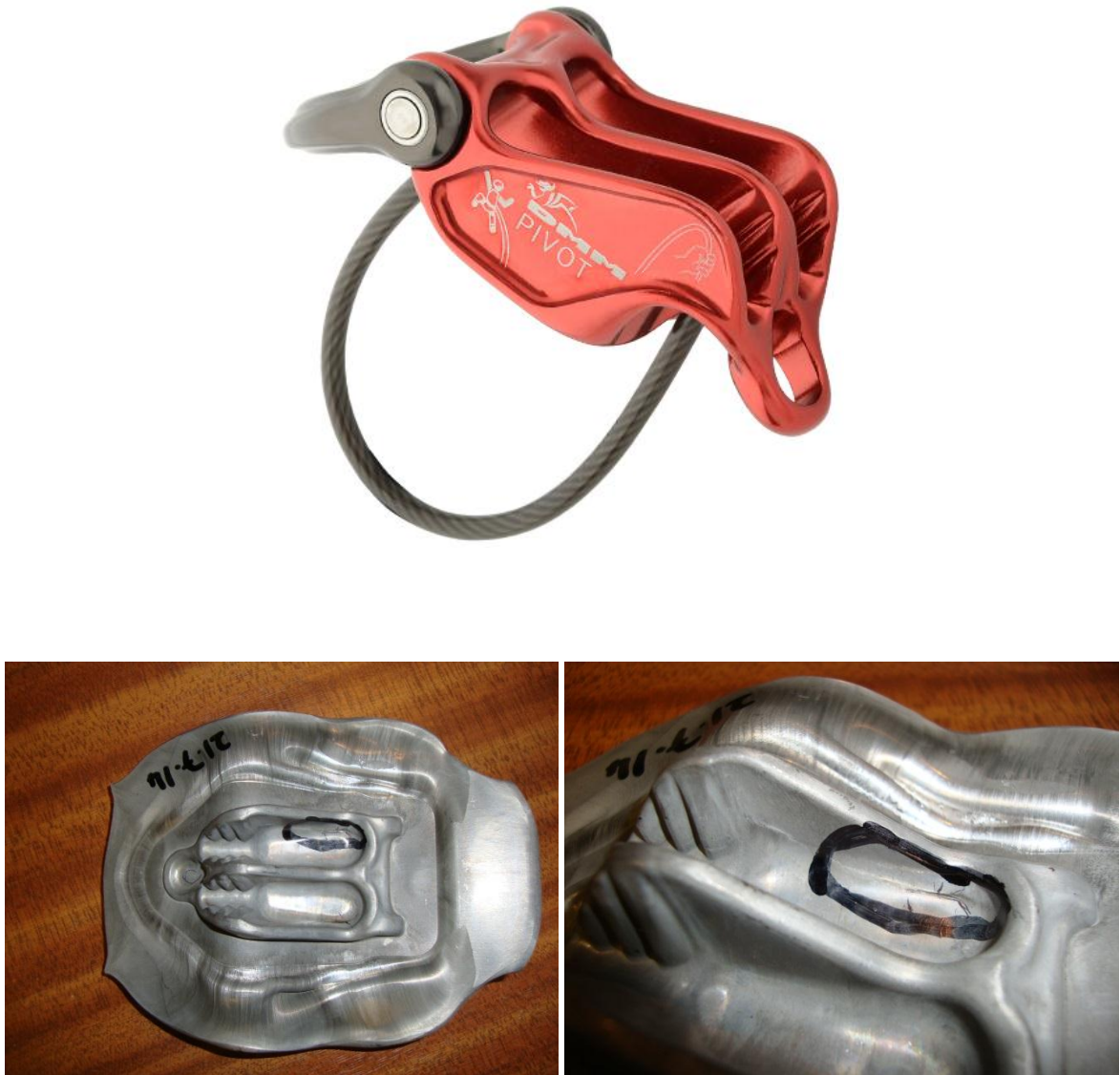
Figure 1. At the top – is the photo of finished part, below – is the photo of the part forged by the initial technology. The defect location in the forged part is circled in black marker (courtesy of DMM)
